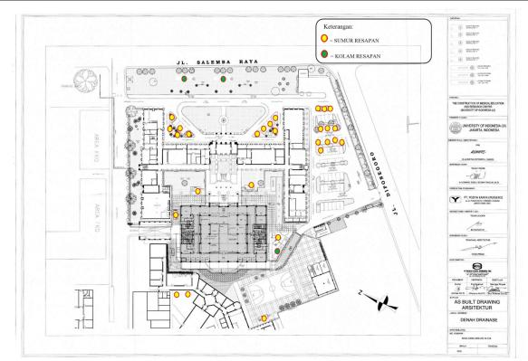
Layout of Infiltration Wells/Retention Ponds at Salemba
